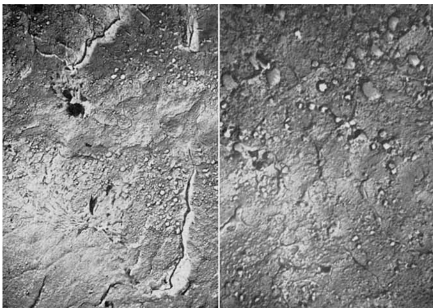
Fig. 11 (left). Fracture surface of PET after 43% weight of crystallization; polymer crystallized at 200°C. 5,000 \times . Fig. 12 (right). Fracture surface of PET after 43% weight of crystallization; polymer crystallized at 200°C. 12,500 \times .
